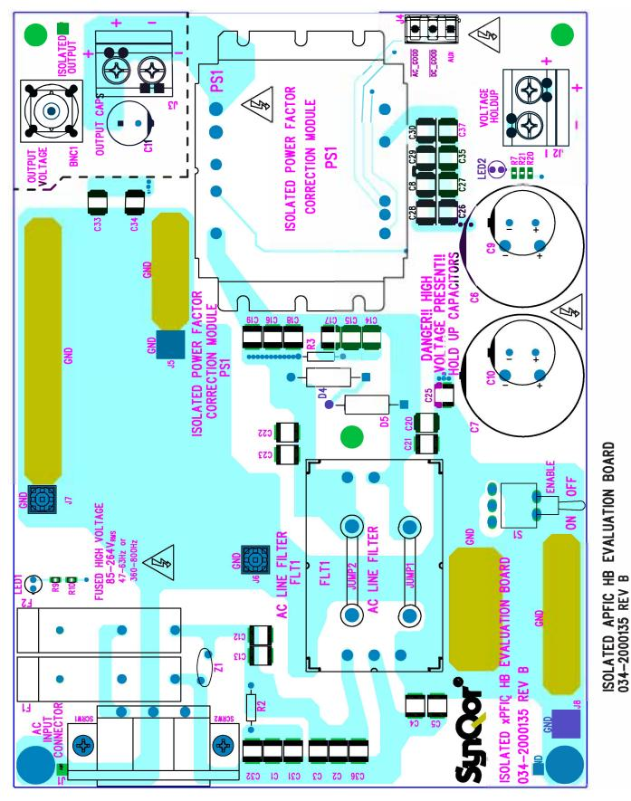
Figure 3: EVAL-1000042 board component placement
